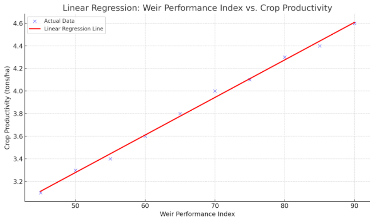
Figure 3. Illustration of Relation Curve between Crop Productivity and Performance Index of Weir.
