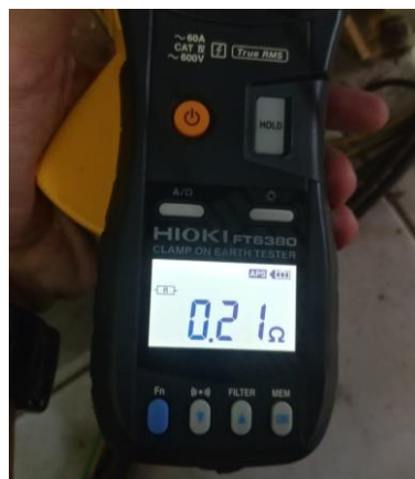
Figure 3. The results of checking the grounding resistance of the testing equipment show a value of 0.21 \Omega .
