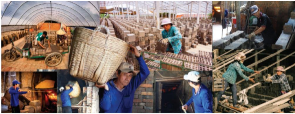
Figure 8: Labor practices in Mang Thít brick and pottery village, encompassing the entire process from clay preparation and molding to stacking, firing, and transportation. These images illustrate the cooperative rhythm and intergenerational transmission of artisanal skills.
